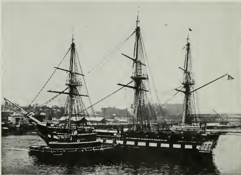
TURN ABOUT— USS Constitution is shown on her annual voyage from mooring in Boston Naval Shipyard as she is turned to keep sun from warping her masts.
